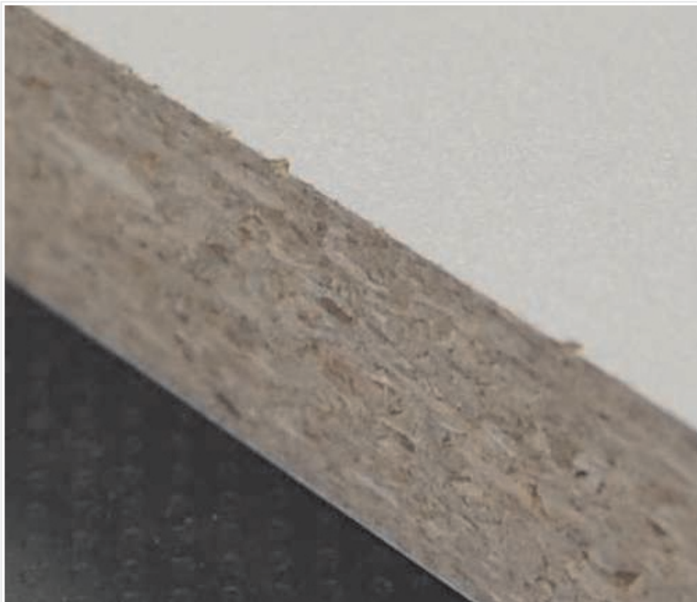
Clean top edge on melamine (top photo), some chip out on the bottom side (bottom photo)
