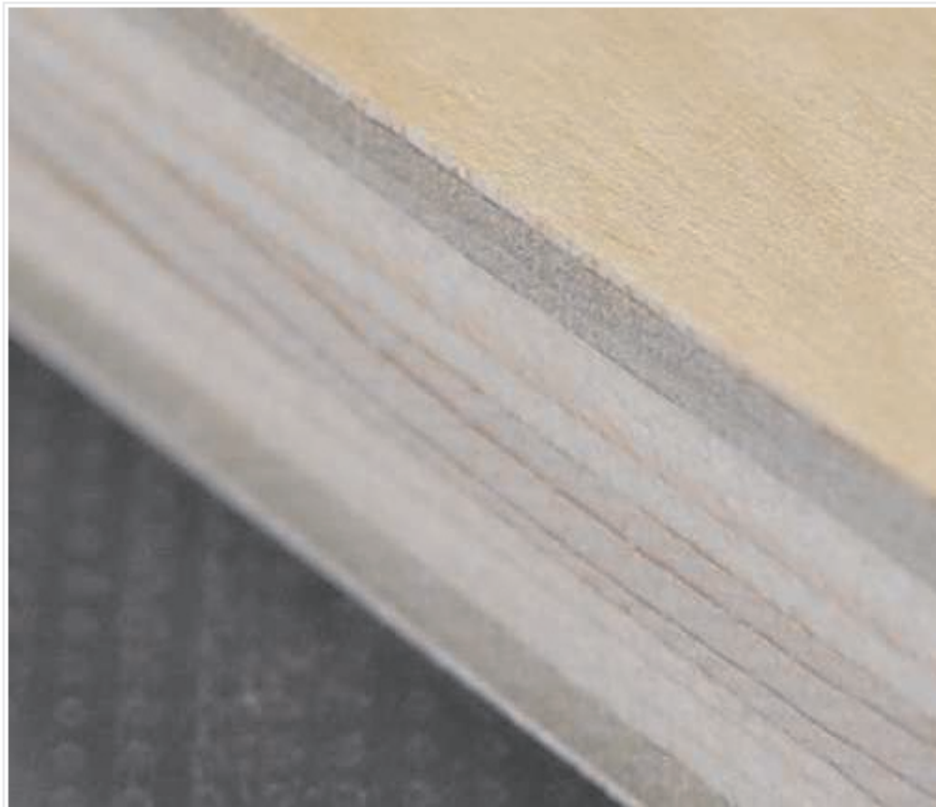
Crisp, clean edges on plywood - top and bottom sides
