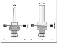
This set is designed to cut slots in wood for biscuit joints, using your Router. By replacing the bearing, you can achieve 3 depths to accommodate the common wood biscuit sizes.
