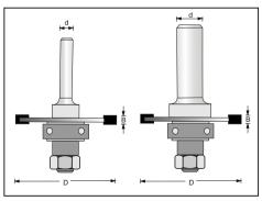
This set is designed to cut slots in wood for biscuit joints, using your Router. By replacing the bearing, you can achieve 3 depths to accommodate the common wood biscuit sizes.
