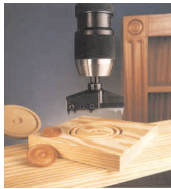
Rosette bit and cutter head require two knives.
