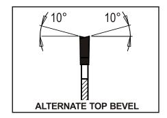
For general ripping and crosscutting along and across the grain of wood, plywood, and particle board. Micro-grain titanium carbide teeth. Non-adhesive black coating. Thick carbide teeth. Premium quality, made in Germany.
