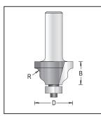
Wavy Edge Bits with Ball Bearing Guide, 2 Flutes
