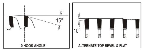
For cutting across and along the grain in wood, plywood, hardboard and particle board. Used in sliding, compound, miter saws and radial arm saws. Micro-grain Titanium carbide teeth. Non-Adhesive black coating. Thick carbide teeth. Premium quality. Made in Germany.
