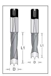
Carbide tipped head with two edges and center point for drilling tear free holes in solid timber or plastic, laminated panel materials. Cylindrical 10mm diameter shank with fixing flat for grub screw and length adjusting screw.
