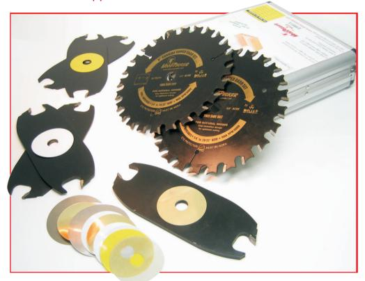
This 8" Carbide tipped safety Dado set will produce flat bottom grooves with splinter free edges in natural woods. Fully versatile, this dado set can be set from 1/4" to 1" widths at 1/16" increments. Micro increments widths are made with the provided shims.
