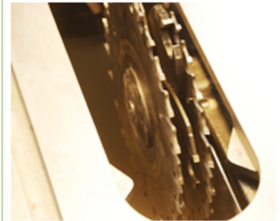
A 1" dado with washer leaves no room for the arbor nut; to install eliminate the washer and install the nut
