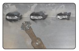
Spot welds: shear off sharp and excess material caused by the molten after brazing or soldering (prior to the finished weld) with a hand-held rotary tool.
