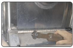
Finished welds: shear off sharp and excess molten material caused by the molten after brazing or soldering (cleaner finished weld) with a hand-held rotary tool.
