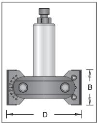
Adjustable Bevel Router Cutter, 2 Flutes
