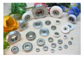
Ball Bearings are one of the most important components in a Router Bit's structure since they have a direct impact on design and performance. Dimar's Deep Groove Ball Bearings have shields installed on both sides and are factory-packed with lubricants. It eliminates the need for relubrication and therefore, reduces maintenance costs. Dimar's selected quality ball bearings have been designed to operate at rotating speeds well above the speeds of the Router Machines on the market.
