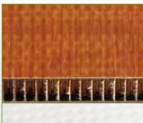
Clean cut using correct tooling
